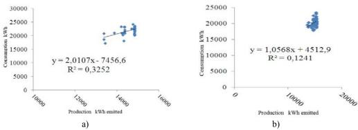
Fig. 3. Correlation Diagram Consumption Vs Production: a) TCMW C; b) TCMW D.
